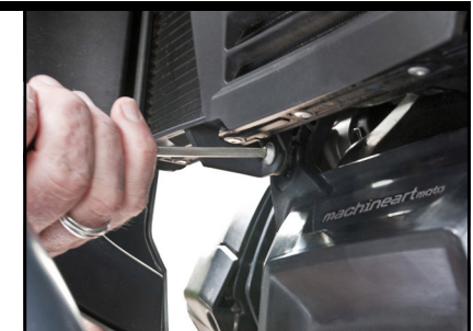
8 Finally, tighten the two T25 Torx screws securing the forked mounting tabs. Check alignment.
