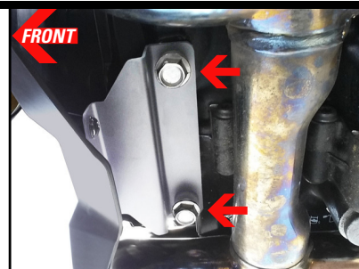
6 Align Hex Bolts with the two threaded holes in the bottom of the engine and start to screw them in by hand.
