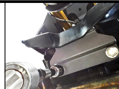
7 Tighten Hex bolts with a 13mm socket wrench.
