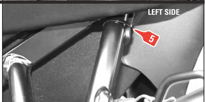
**6** On the right side of the bike, feed the zip tie from the bottom side, up through the backside hole of the MudSling until you see it come out from behind the square tubing. Pull it out, feed it through the front hole, cinch it up securely and trim off any excess length.
