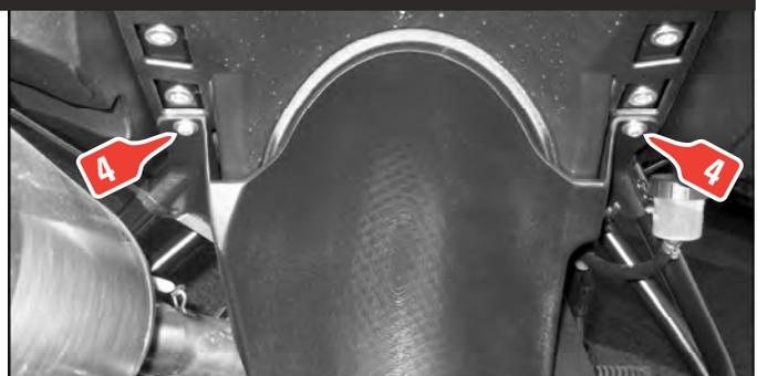
**4** Install the two longer TORX head screws provided with rubber washers. *Loctite is not compatible with ABS plastic. If you do use it, sparingly apply only QUICKSTIX 248.*
