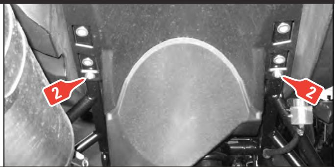
**3** From the right side of the bike, position the MudSling securely against the underseat area, aligning the holes of the MudSling with the holes of the screws just removed. When positioned correctly the widest part of the MudSling will rest against the frame rails that support the footpegs.
